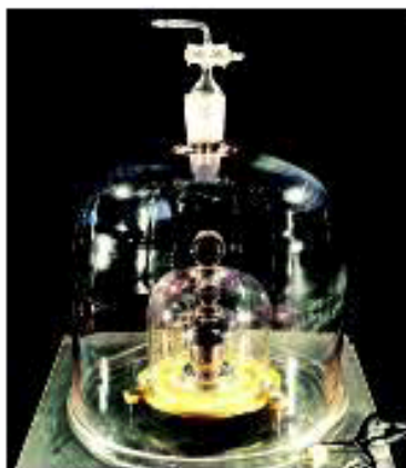
The international prototype of a kilogram. Its mass has changed by a grain of sand
